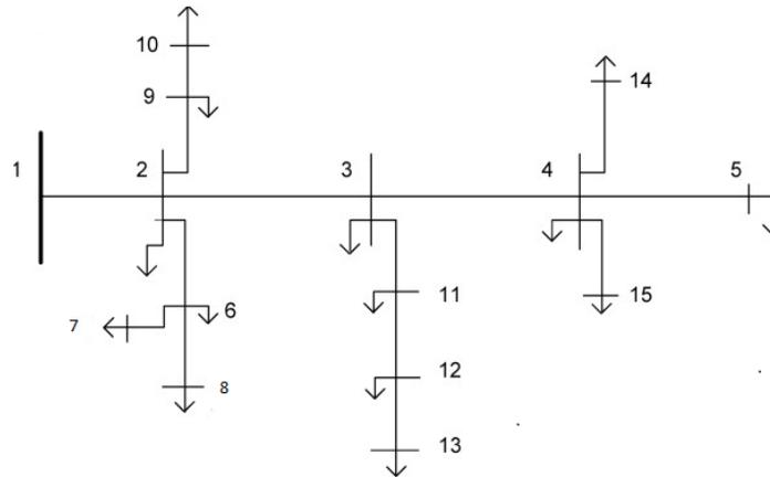
**Figure 1: Radial Distribution Networks for 15 Nodes**
