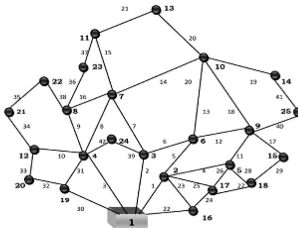
**Figure 2: Graph of Available Supply Routes for 25 Load Nodes Distribution Network**
